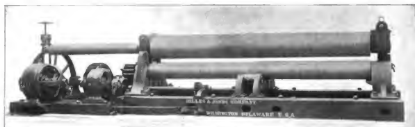
Fig. 4888. Heavy Plate Bending Rolls, Provided with Two Motors. One for Driving the Lower Rolls and the Other for Raising and Lowering the Top Rolls. Hilles & Jones Company.
